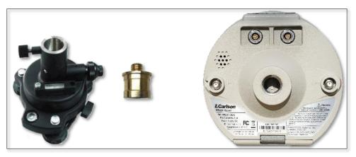
Figure 15: Tribrach Installation Parts
