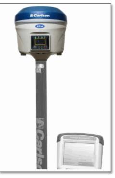
Figure 19: Range Pole Installation
